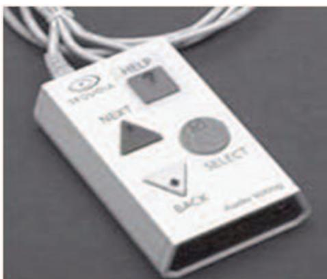
The picture to the left shows a different tactile keypad layout on an accessible voting system. This keypad has only a forward/next key, a back key, and a select key (similar to a switch with three activations.) These buttons are different sizes and colors to support easy differentiation.
