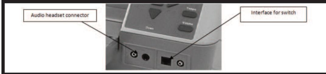
Accessible voting systems that do support switch input typically come with at least one dual switch. Almost all systems are set up to use a dual switch (A/B type input). Thus the types of switches that can be used include just about any dual switch such as:
